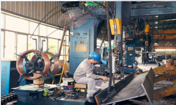
重型雙絲懸臂埋弧焊 (submerged arc welding)
