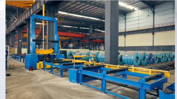
H型钢组立机 (H-shaped steel assembly machine)
