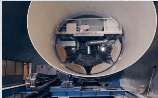
環氧粉末噴塗機 (epoxy powder spraying machine)
