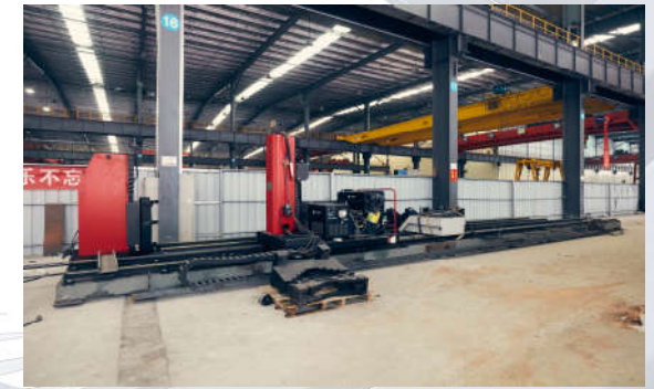
相貫綫切割機 (Intersecting line cutting machine)
